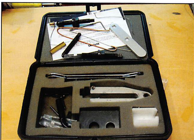
photo.5 - This is the Lockmasters Neutralization Kit. It contains a wide variety of tools used to open and service safe deposit locks. It also has a few home-made tools included in the kit.
