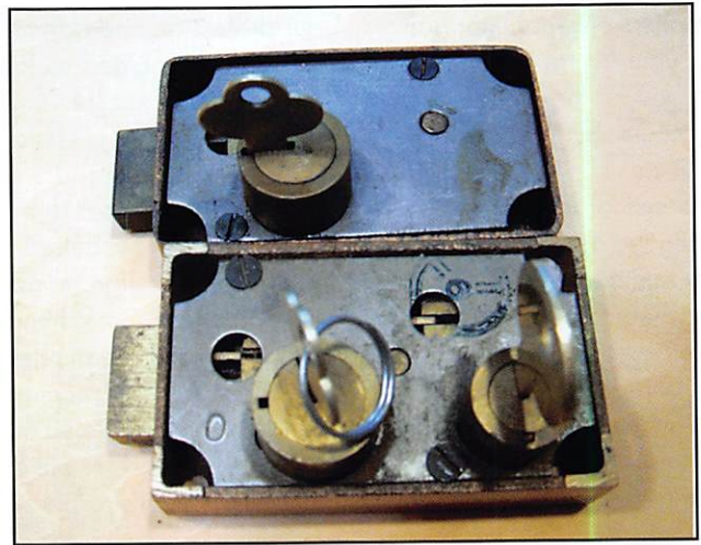
photo.1 - Here are two different same footprint or size one with a single nose and the other having two noses.
